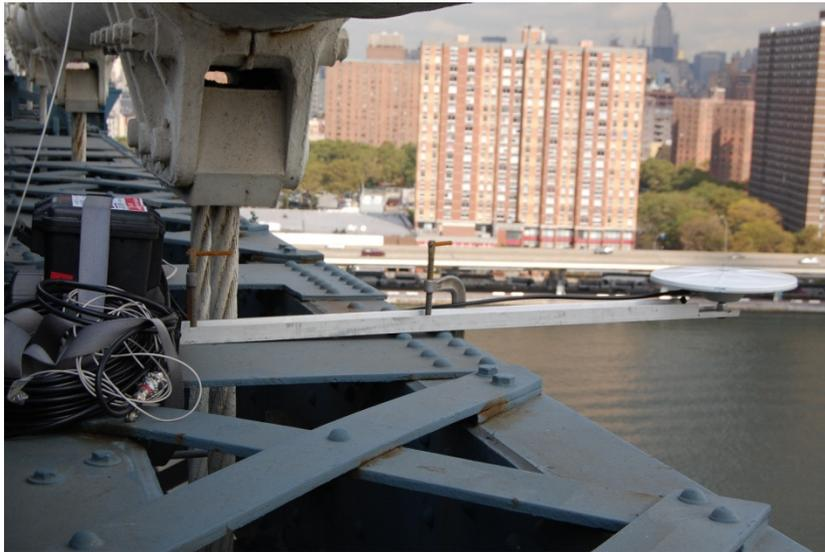
**Figure 4. GPS receiver mounted on Manhattan Bridge**
